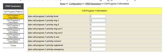
The example below shows an output set to activate during ring (pattern 2), or when a call is connected, or when the telephone is registered.
